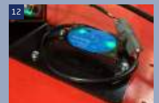
12 Angle sensor: when it is lifting and walking on the slope, the sensor will automatically judge the status of the machine, if the angle is larger than the rated angle, it will alarm to remind the operator.
