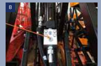
8 Explosion proof valve: To prevent the machine falling when the oil pipe is leaking
